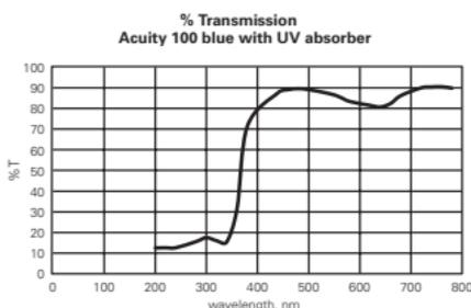
Acuity 100™ (hexafocon A) Contact Lens - Spectral transmittance curve for Acuity 100™ (hexafocon A) Contact Lens - D & C Green No. 6 and UV absorbing agent (sample thickness Acuity 100™ (hexafocon A) lens thickness = 0.12mm)
